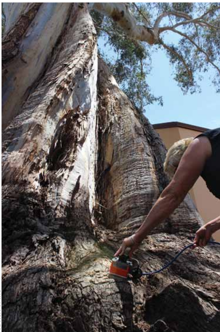
A technician using the Palm 2000 antenna during a Level 3 inspection.
